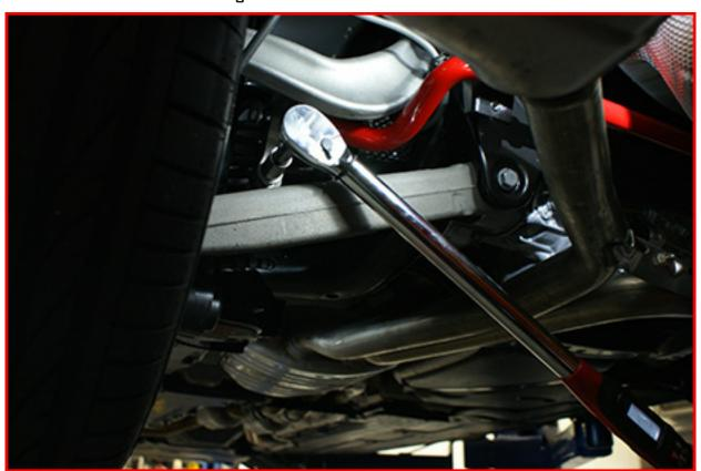
Torque both XZN 10MM triple square bolts to 25Nm (18.4 ft/lb) plus an additional 90 degree (1/4) turn, do this for both sides, ensure you torque evenly.
