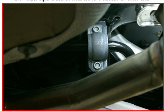
Remove sway bar from vehicle, separate the sway bar bushing bracket from the bar and place bar in a safe area. Repeat on other side.
