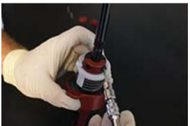
Your Meisterwerk ASTS is now ready for installation into vehicle. Place shifter inside the shifter housing (as pictured) and lower until bearing retainer is touching the shifter housing. Line up the shifter so that the bearing retaining clips and bearing housing can be screwed together with the two socket cap screws removed in step 10.
