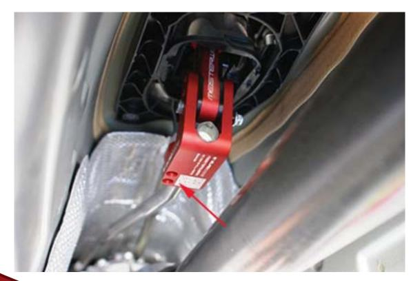
Temporarily replace the factory shifter surround back onto the center console and place the shift knob and boot assembly onto the shifter. Check to make sure the shifter is centered from left to right and front to back. If the shifter appears to be centered, go underneath the vehicle and torque the two cap screws 40 in/lb (do not over tighten). If the shifter needs adjustment front to back, go to step 20.
