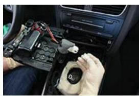
Remove foam sound insulation and rubber weather seal from the shifter base. The rubber weather seal is held in place with two small tabs towards the back. The lower left photo shows you where to pry. Gently pry tabs away from shifter base as shown in the upper right photo and lift up and to the rear of the vehicle as shown in the lower right photo.
