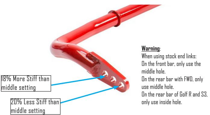
**Warning**: Make sure both rod ends are installed in the same hole location on either side of the swaybar. Also, these settings affect the handling characteristics of the vehicle. Make sure, when testing different settings, to drive the car in a safe and controlled environment such as on a race track. Always drive safely and follow all traffic laws on public roads.
