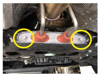
Remove the two bolts of the pendulum support from the engine. (16mm socket)
