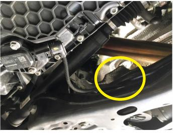
Remove the two bolts to detach the steering rack from the subframe. Pry the steering gear out of the subframe alignment sleeves. (18mm socket)
