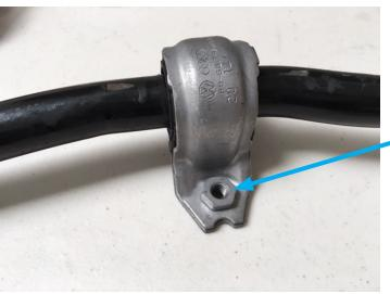
Remove the nuts to separate the brackets
