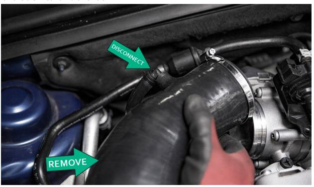
Keep the larger work clamp on the intake side of the intake inlet for re-installation of the new inlet. You will not need the smaller clamp on the throttle body side.
