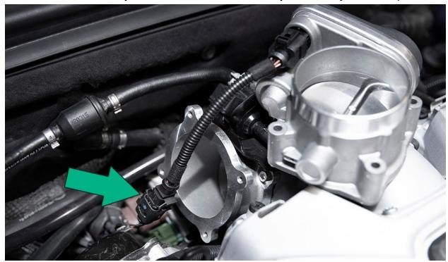
Install the two provided long (50mm) allen bolts into the top of the new throttle body with the new 80mm gasket to the throttle body adapter. Hand tighten bolts with a 5mm allen.
