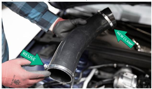
Install the new intake inlet silicone into place adjusting the position of the intake silicone making sure it is not pulling or bound and that it sits freely without tension. Firmly tighten both hose clamps with a phillips screwdriver. **Do not over-tighten clamps.**
