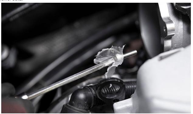
Once all bolts are hand tight, tighten all 4 bolts firmly with 5mm ball end allen.
