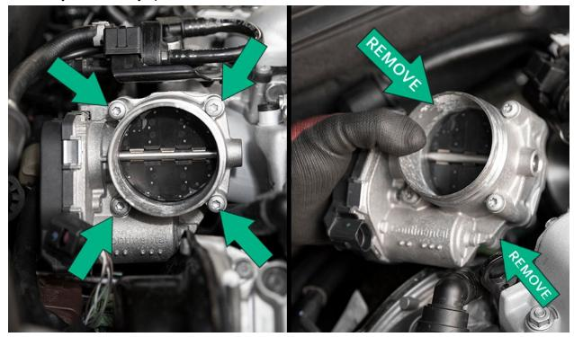
Your new throttle body setup will be much larger, to accommodate the increase in size you will need to bend up the purge valve bracket located above the throttle body location. This is a soft metal and can be done by hand.
