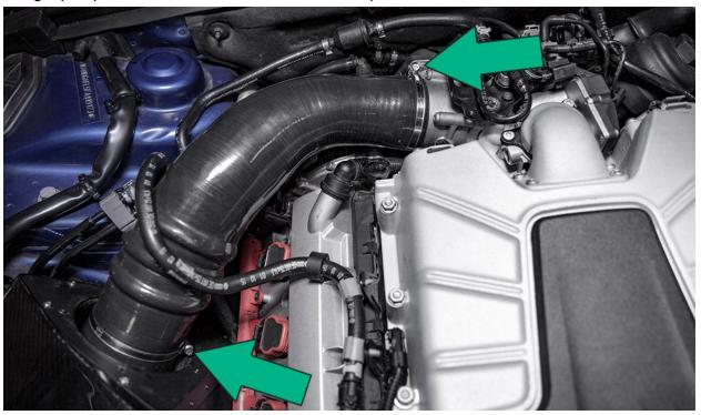
Remove the factory breather line from the 90-degree hose barb in the intake inlet silicone, and remove the inlet from the vehicle.
