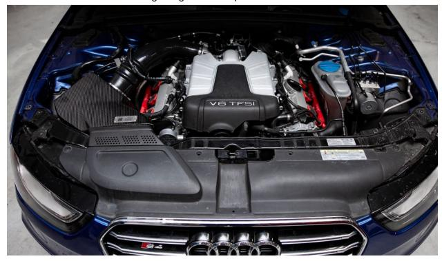
Carefully pull up on the corners to release the clips and remove the rear engine cover plastic. (If you want to reinstall this part with the new throttle body, it will require custom modification.)
